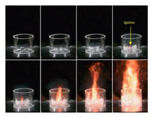
The propellant developed at Łukasiewicz – ILOT is a safer alternative for personnel and the environment to the toxic materials currently in use – hydrazine derivatives and nitrogen oxides. The developed combination uses hydrogen peroxide (with a concentration of 98%) as oxidizer with a novel fuel.
