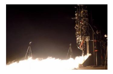
This was the LPL's first successful test fire of a regenerativelycooled engine and one of the few successful ones to date in collegiate rocketry. The student group additively manufactured this engine by laser powder bed fusion with the help of its industrial partner i3DMFG. LPL will test-fire this engine again later this year, introducing adding important thrust vectoring capability.
